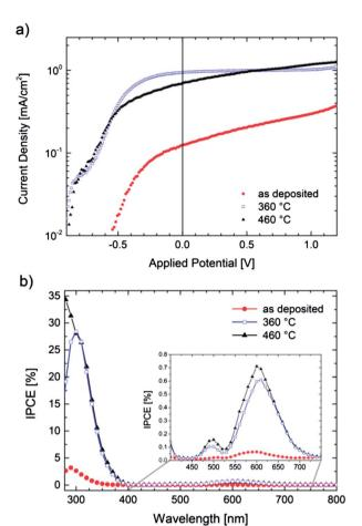
Fig. 5 (a) I-V characteristics of TiO<sub>x</sub> films (scan rate 2 mV s<sup>-1</sup>) under illumination (375  $\mathrm{mW}~\mathrm{cm}^{-2}$ ) and (b) quantum efficiency (IPCE) at  $U_{\rm appl} = 0 \text{ V}.$
