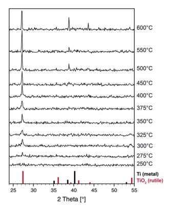
Fig. 4 In situ  $\theta$ – $2\theta$ -XRD measurement of a TiO<sub>x</sub> film (p(O<sub>2</sub>) = 0.2 Pa during deposition) and powder patterns of TiO<sub>2</sub> (rutile structure, PDF file 21-1276) and metallic titanium (PDF file 44-1294). The slight shift of the experimental peak positions relative to the TiO<sub>2</sub> pattern is due to small changes in the diffraction geometry during heating.
