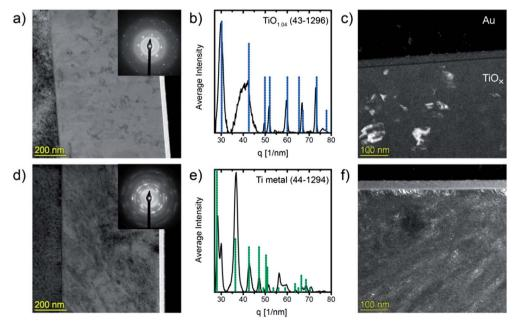
Fig. 3 Cross-sectional TEM-micrographs of TiO<sub>x</sub> films: (a) BF-TEM and (c) DF-TEM of pristine TiO<sub>x</sub>, (d) BF-TEM and (f) DF-TEM of a film that was annealed at 360 °C. Insets in (a) and (d): SAED patterns of the films. (b and e) Circularly averaged intensity distribution of the SAED pattern and corresponding phases. During preparation of the FIB lamellae the films were coated with an amorphous carbon layer and gold contacts.
