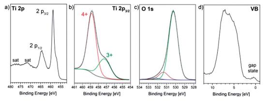
Fig. 1 (a) XPS detail spectra of the Ti 2p signal, (b) fitted Ti  $2p_{3/2}$  and (c) O 1s lines; (d) X-ray induced valence band spectrum of a TiO<sub>x</sub> film that has been deposited under  $p(O_2) = 0.2$  Pa.
